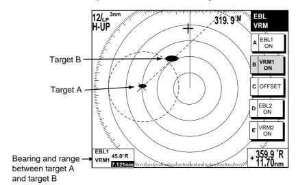
Measuring range and bearing between two targets
